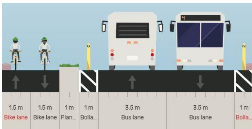
Figure 4-8: Indicative cross section BRT (13m dual lane)
